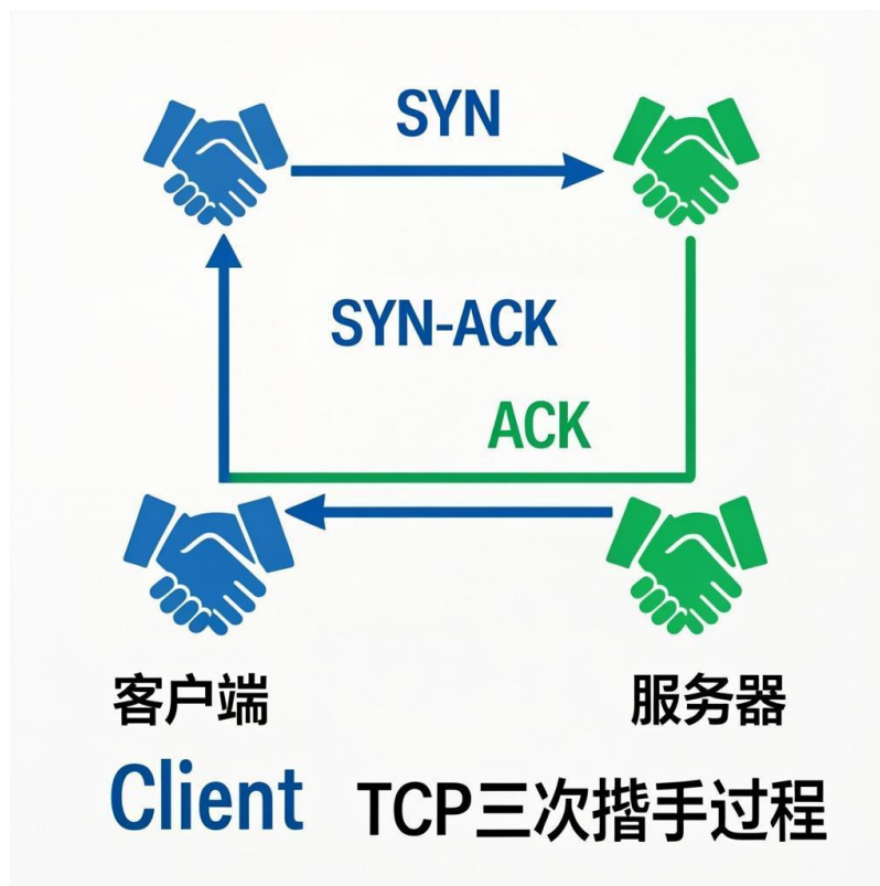
Figure 1 : Le Three-Way Handshake TCP
